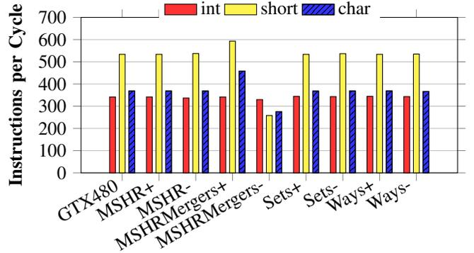
Figure 7. Performance potential behind various cache and memory fetching resources. *MSHR*, *MSHRMergers*, *Sets*, and *Ways* indicate a change in number of MSHR entries, MSHR merger entries, L1 sets, and L1 ways in set, respectively. + or - indicate 2X higher or lower resources, respectively.
