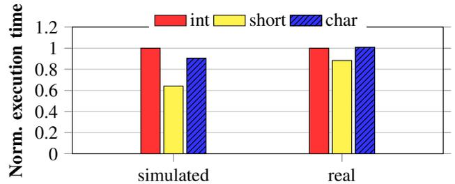
Figure 4. Normalized execution time of 1D stencil under real/simulated GTX 480 and different data types (int, short, and char are 4-, 2-, and 1-byte per element).
