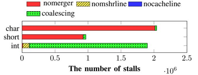
Figure 6. Breakdown of stalls under 1D stencil for different data types.
