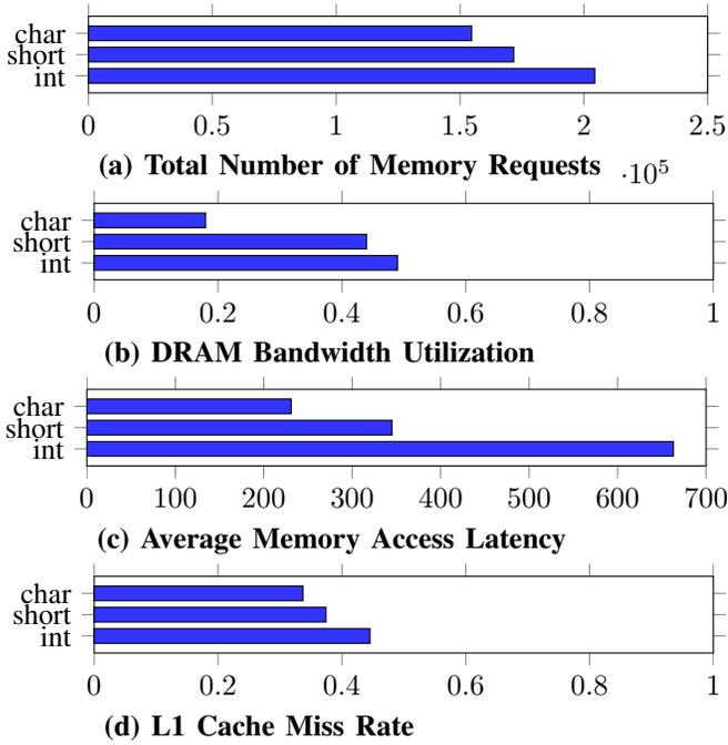
Figure 5. Memory efficiency metrics under different data types for 1D stencil.
