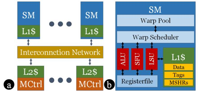
Figure 2. (a) High-level design of a GPU chip. (b) microarchitecture of SM.
