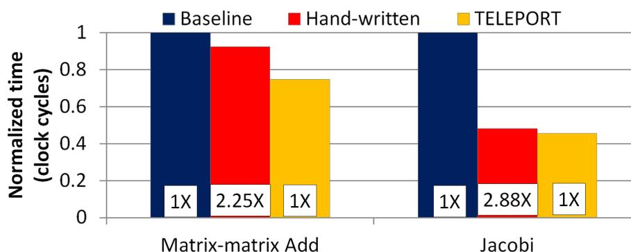
Figure 7.1: Comparing three different implementations of Matrix-matrix Add and Jacobi iteration. Bars report kernel time and numbers below the bar indicate the development effort, normalized to Baseline. (Effort is measured in the number of lines of code.).
