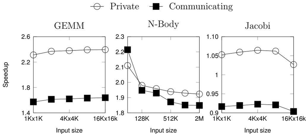
Figure 5.6: Comparing speedup from different renewing cache scope methods. Numbers are normalized to the baseline OpenACC without using the cache directive.
