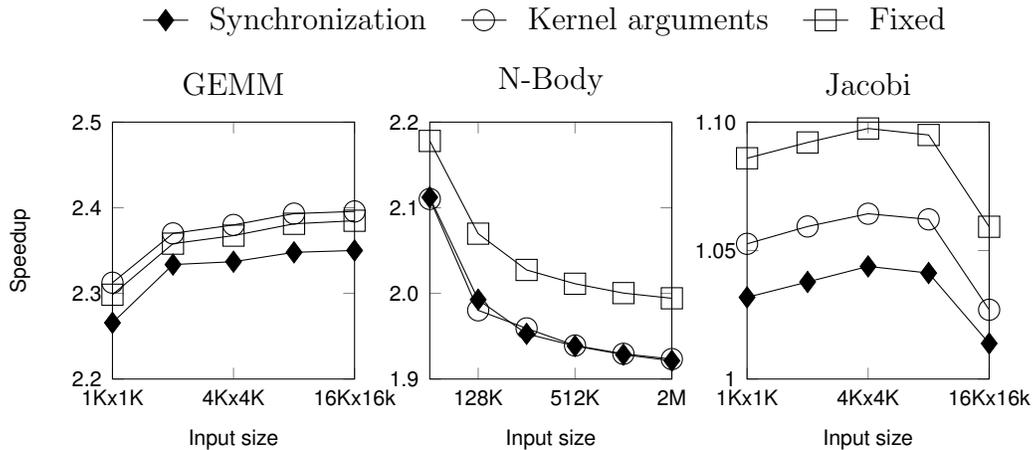
Figure 5.5: Comparing speedup from different finding sharing width methods. Numbers are normalized to the baseline OpenACC without using the cache directive.
