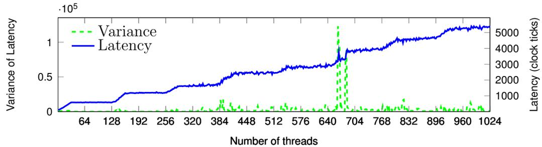
Figure 4.9: Thread-Latency plot under Tesla K20, two loads per thread, and Two-coalesced memory pattern.
