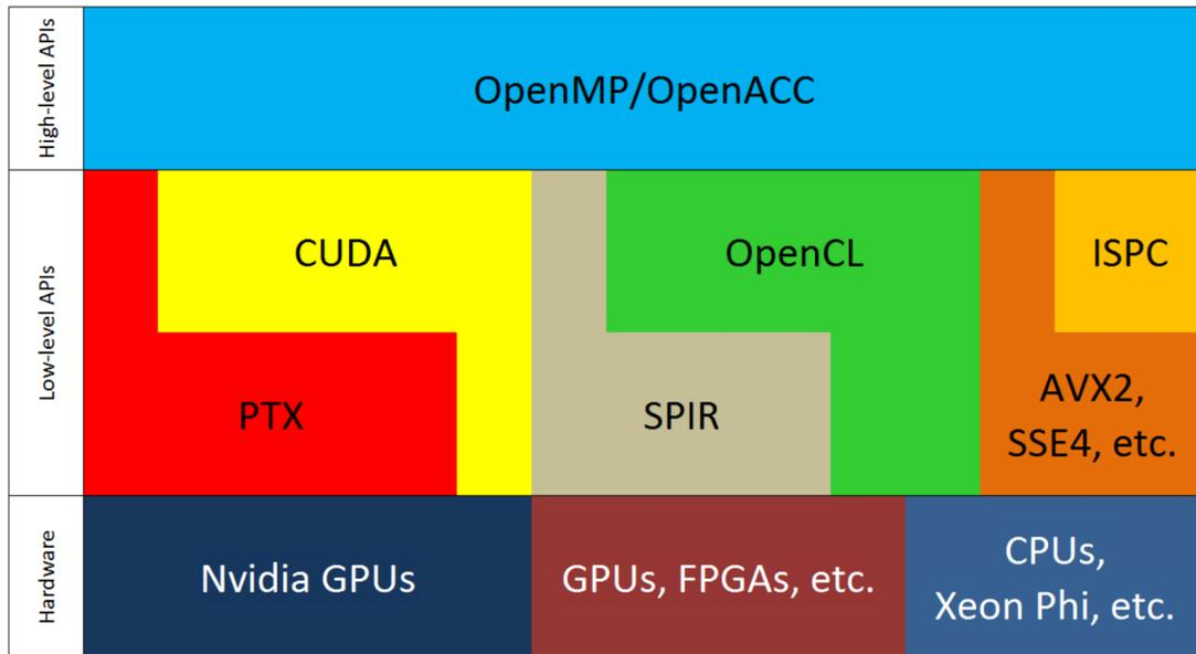
Figure 2.1: Hardware and software stack of accelerator-based computing.
